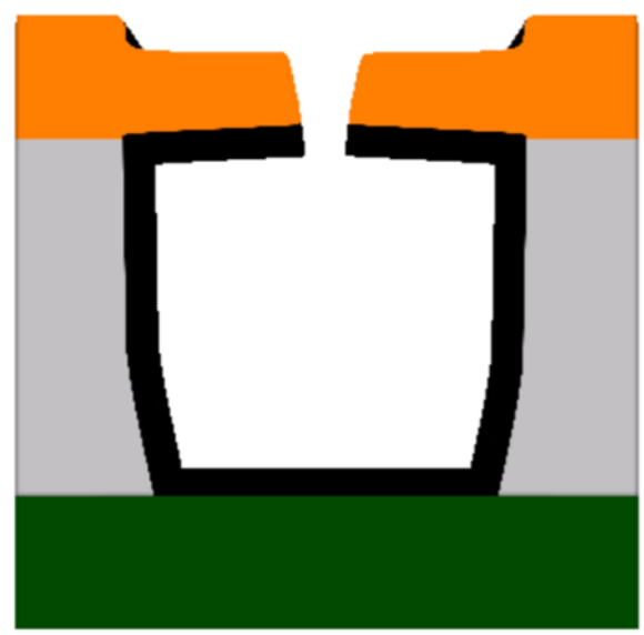
Resist profile of Niemeyer-Dolan Bridge
