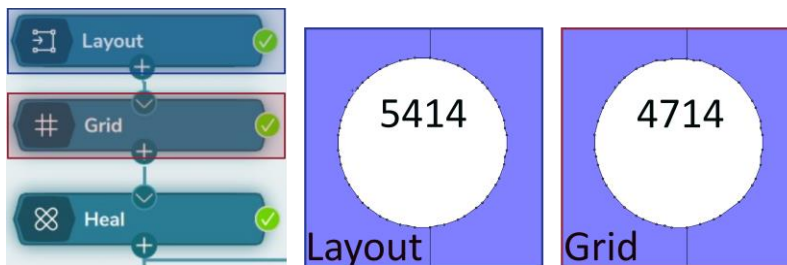
Figure 5. (left) Import, Grid and Heal modules, (middle) imported layout with 5414 vertices, and (right) layout after grid module with 4714 vertices.
