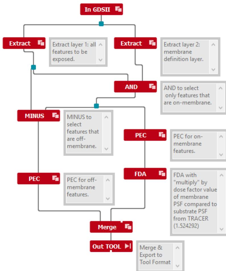
Figure 6. Sample BEAMER flow for membrane dose assignment.
